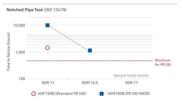
$NOTE: Test\ covered\ 110mm\ pipes\ with\ notch\ depth\ of\ 2.1mm\ tested\ in\ hydrostatic\ pressure\ test\ at\ 920kPa/80°C$
